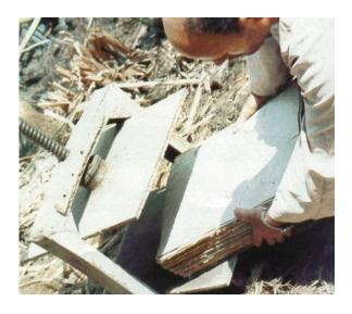
The whole block is clamped in a press and then left in it for 12 hours under constant pressure. During this process, the individual strips are joined together by the remaining sugar to form the papyrus sheet. After the pressing process, the sheets are again placed between drying felts to remove the remaining water. The sheets are also put back into the press for about 12 hours.
