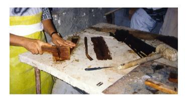
In contrast to the production of natural papyrus, the cooked pieces are now beaten flat with wooden mallets or hammers. For this reason, more raw material is required for the production of antique papyrus. In order to avoid mutual sticking, the individual sheets are placed on air- and waterproof foils and then pressed.
